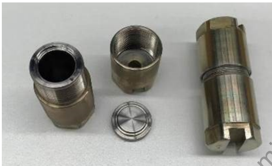
Figure 2: Micro autoclaves used in the batch experiments
